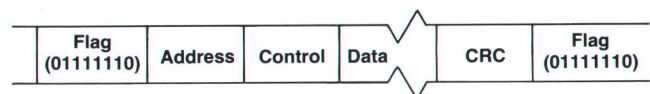
Fig. 4. Format for SDLC message. The 01111110 flag pattern is used to synchronize messages.
