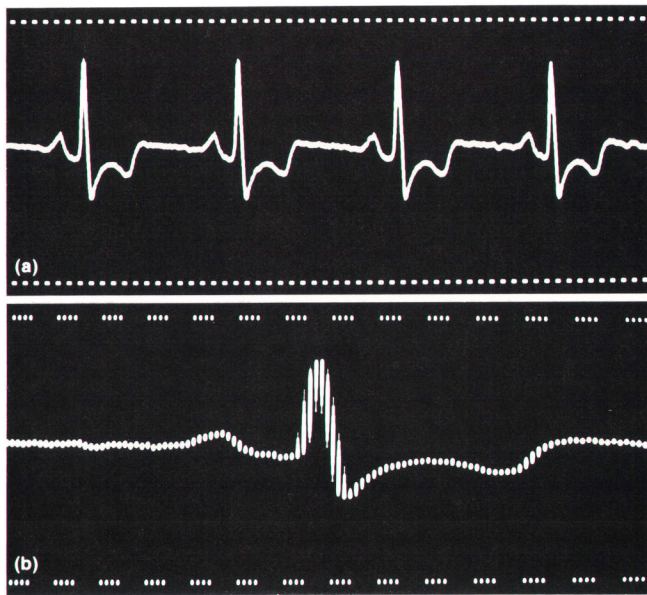
Fig. 2. (a) Photo of a normal waveform as shown on the 78510A Display. (b) Expanded view of waveform in (a) showing video modulation required to display waveform.
